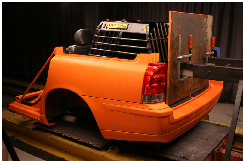
The plate enters the luggage compartment just a little bit above the floor and push the crate forward during the braking of the crash test sled.
