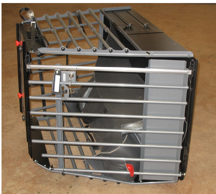
The Variocage crate after the drop test was resting on its side.
