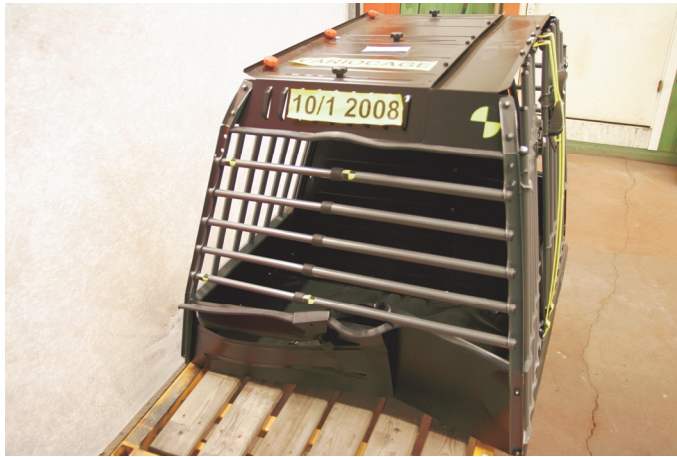
The crate was compressed approximately 150 mm. No sharp edges could be found.
